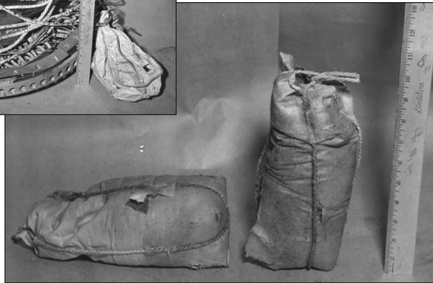
The altitude control mechanism (left) and two sandbags recovered from the Japanese balloon that landed near the lower Yukon River community of Marshall on December 23, 1944. Note the empty sandbag attached to the control mechanism. Photographs courtesy of the National Archives and Records Administration, College Park, Maryland. (Box 42, RG 499)
