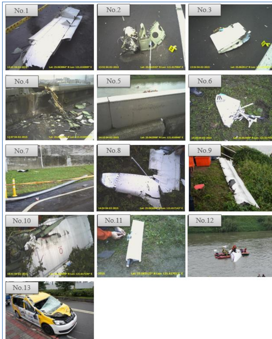
Figure 1.12-3 Site survey- wreckage identification numbers and photos.
