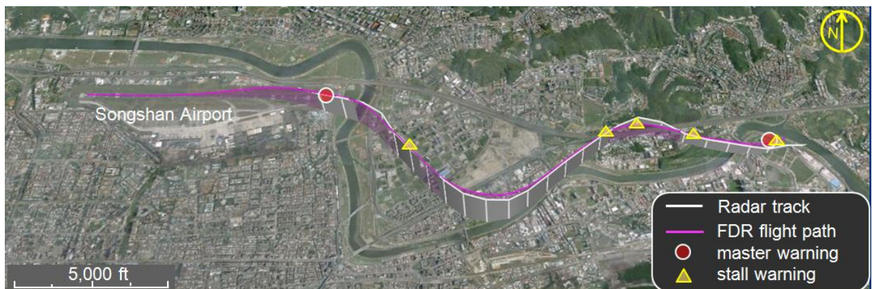
Figure 1.11-8 Superposing of GE235 flight path, radar track and warnings
