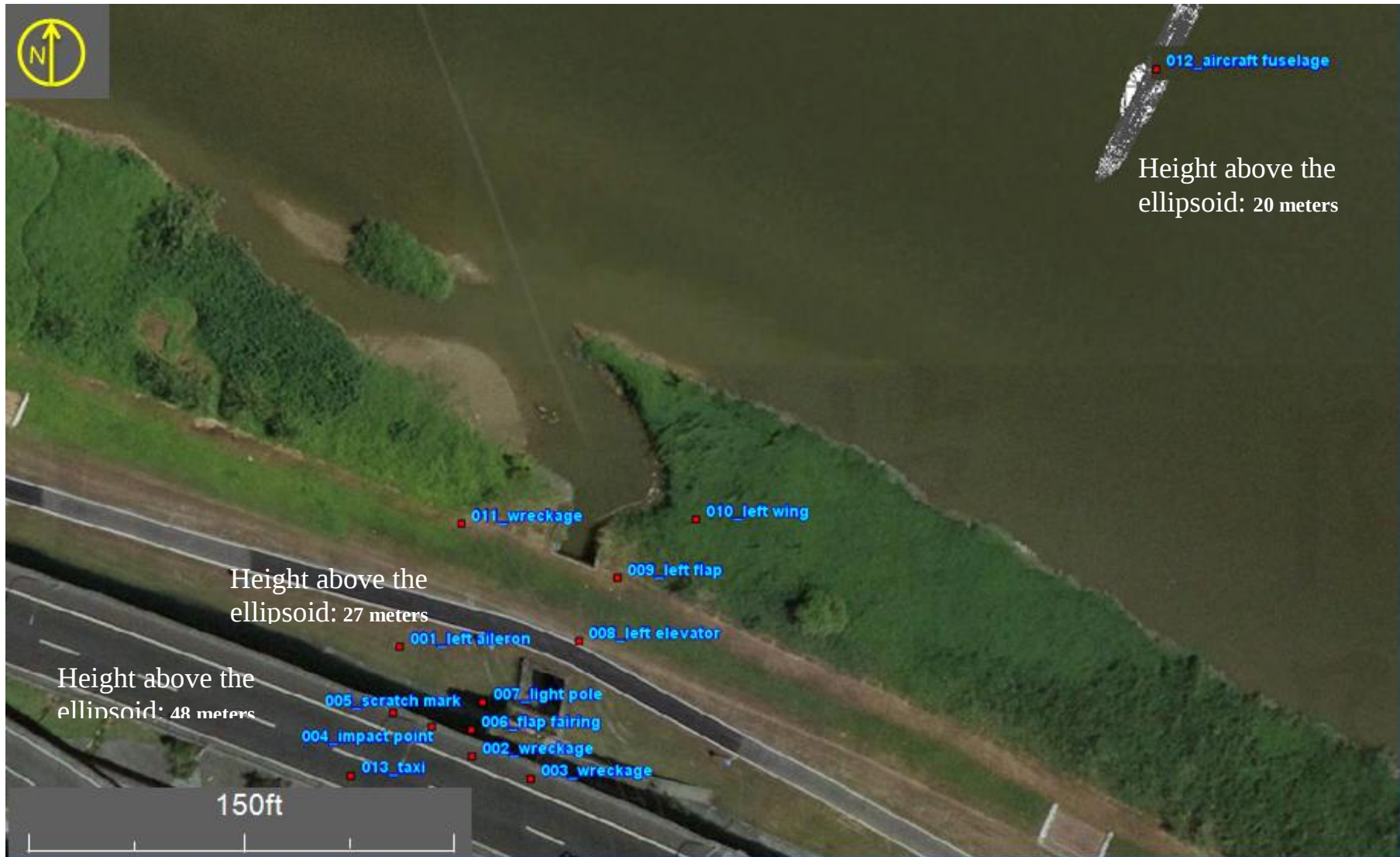
Figure 1.12-2 Site survey data superposing with an aerial photo
