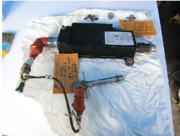
Photo No. 22 Autofeather unit and torque sensor No. 1.
