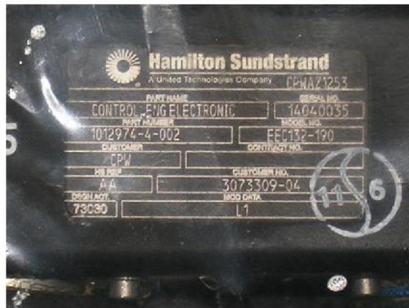
Photo No. 21 Engine electronic control data plate.
