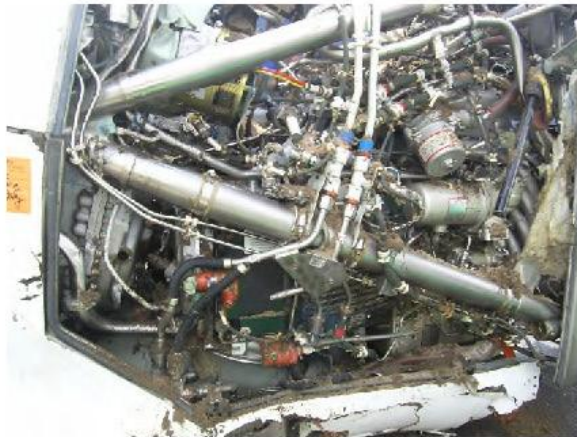
Photo No. 35 Compressor inlet case, Autofeather unit and engine electronic control, in-situ.
