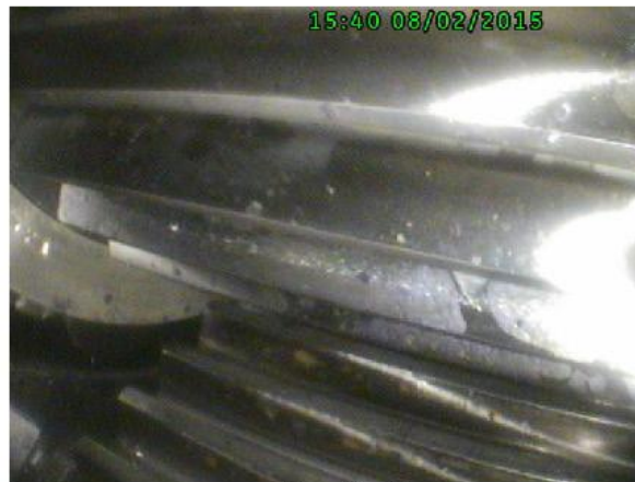
Photo No. 15 Reduction gearbox second stage spur gears, detail.
