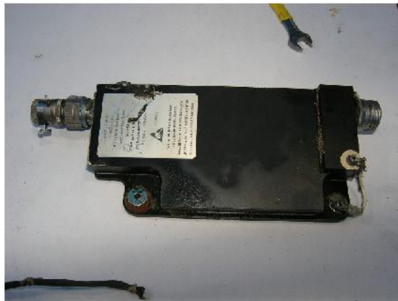
Photo No. 53 Autofeather unit.
