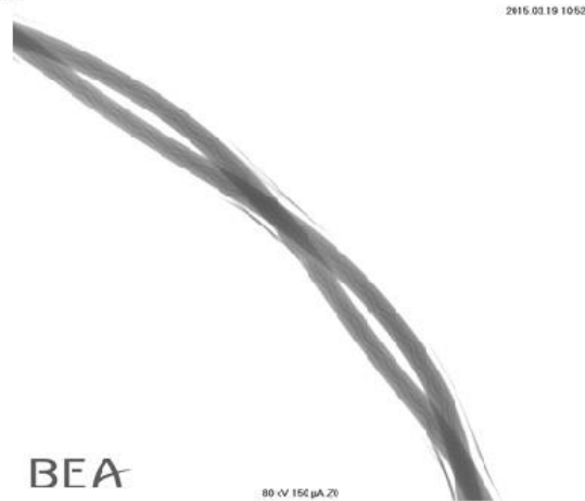
Figure 6: typical RX picture of the cable between the 2 connectors
