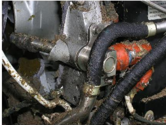
Photo No. 58 Torque sensor No. 1, in situ.
