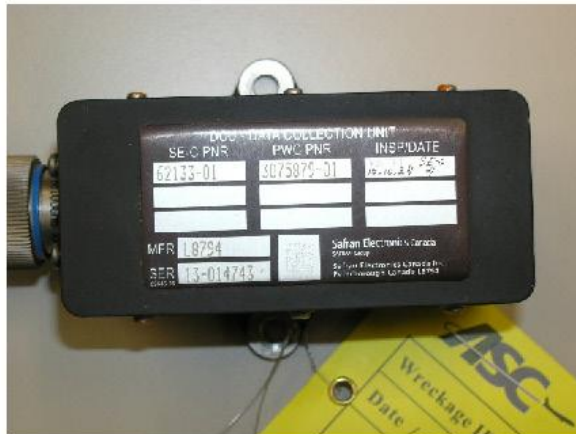
Photo No. 57 Data collection unit data plate.
