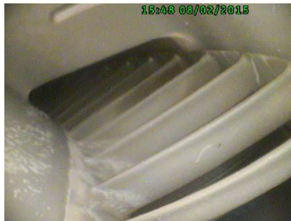
Photo No. 40 First stage power turbine vane ring.
