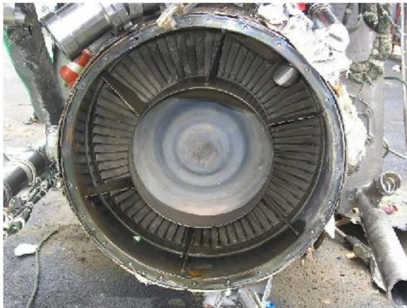
Photo No. 37 Exhaust duct and power turbines.
