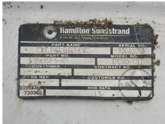
Photo No. 50 Propeller electronic control data plate.
