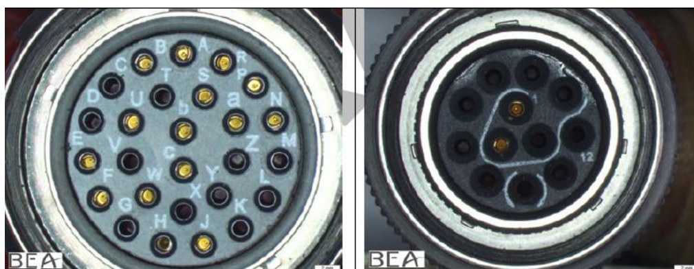
Figure 1.16-6 Torque sensor and AFU connectors
