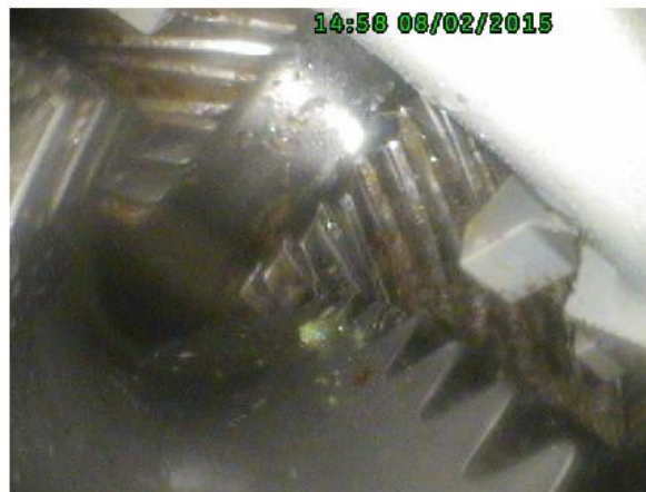
Photo No. 47 Reduction gearbox helical input gearshaft and helical gear.
