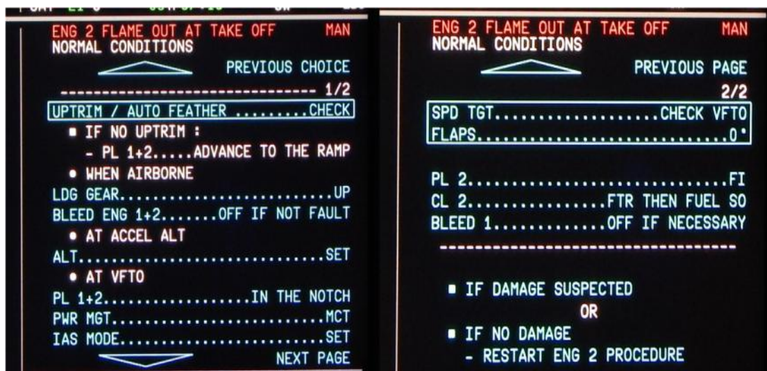
Figure 1.6-4 Simulated EWD display of ENG 2 FLAME OUT AT TAKE OFF procedure
